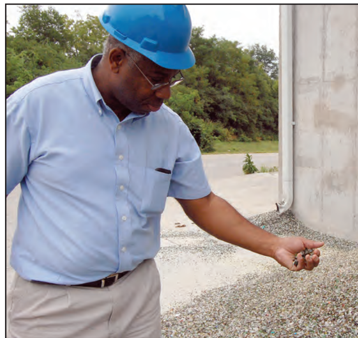
Above: Recycling truck driver Ernie King takes a last look at Tuesday's glass haul from Berea at Bluegrass Regional Recycling in Lexington. At left: plant manager James Carter demonstrates that the glass is safe to handle after it has gone through the line. It's broken up in the hopper by many little hammers which rounds the edges of the glass making it safe to handle.
